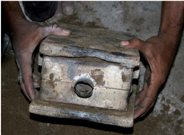
Fig. 1 Metal sand casting flask, length c. 25 cm (above) and assembled with front and back boards, showing ingate (below), for casting of bidri ware in modern Hyderabad, India.
